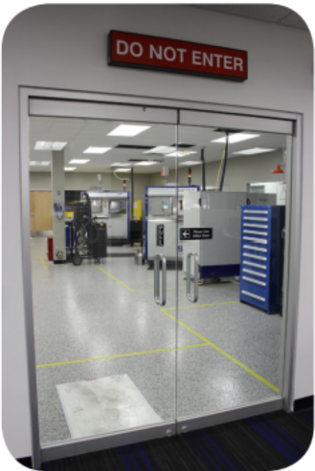
Secure entry with signage and tack mats inside the lab door prevent powder contamination outside of the machine area
